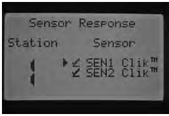
Both sensors programmed for Station 1
